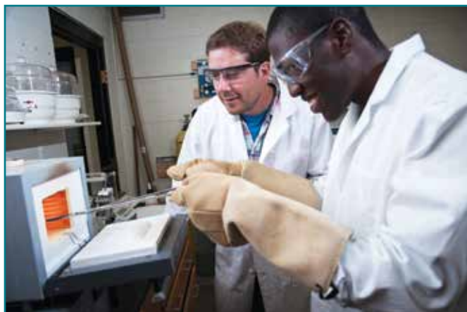
PAUL GANNON (left), faculty advisor of the new ECS student chapter at Montana State University, observes as JUDE EZIASHI removes a high-temperature corrosion specimen from a furnace system.
