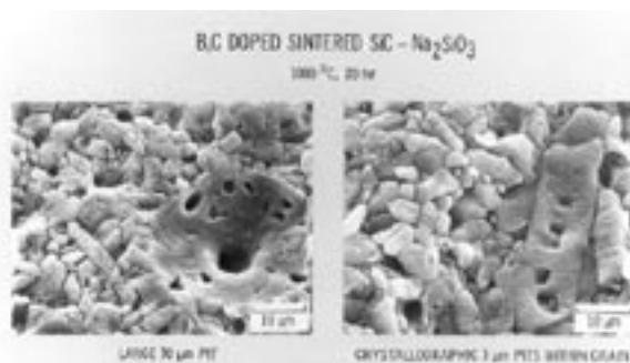
Fig. 3. Photomicrographs illustrating pit formation during oxidation of sintered SiC in a combustion atmosphere. A mechanism explaining the formation is given in Fig. 2 (Courtesy of N. Jacobsen and J. Smialek at NASA Glenn Research Center.)
