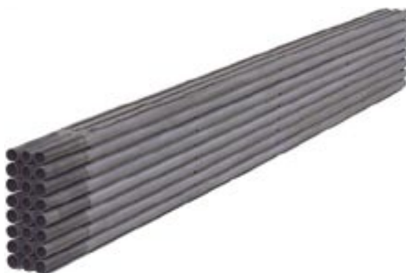
Fig. 1b. Schematic diagram of a SOFC bundle configuration. (Fig. 1a and b courtesy of Siemens Westinghouse Power Generation.)
