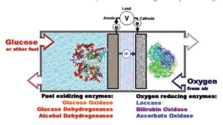
**FIG. 1.** Generalized schematics of an enzyme biofuel cell consisting of an anode, catalyzed by oxidases suitable for conversion of fuels of choice or a complex of such enzymes for a complete oxidation of biofuels. The cathode usually features an oxidoreductase that uses molecular oxygen as the ultimate electron acceptor and catalyzes reduction to water in neutral or slightly acidic media.
