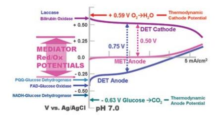
**FIG. 2.** Principles of biofuel cell design indicting the maximum oxidation potentials for glucose and the corresponding thermodynamic potential for oxygen reduction at neutral pH. Redox potentials of several enzymes and their corresponding co-factors are shown along with the potential "zone" containing the redox potentials of the usual mediators. Polarization curves depict typical current performances for direct and mediated electron transfer in biofuel cell electrodes.
