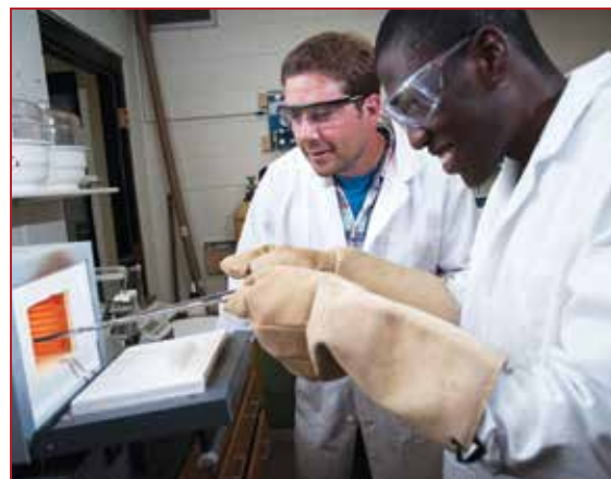
PAUL GANNON (left), faculty advisor of the Montana State University Student Chapter , observes as JUDE EZIASHI removes a high-temperature corrosion specimen from a furnace system.
