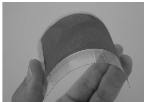
Fig. 1 Flexible plastic film photoelectrode bearing dye-sensitized mesoporous TiO 2 layer
